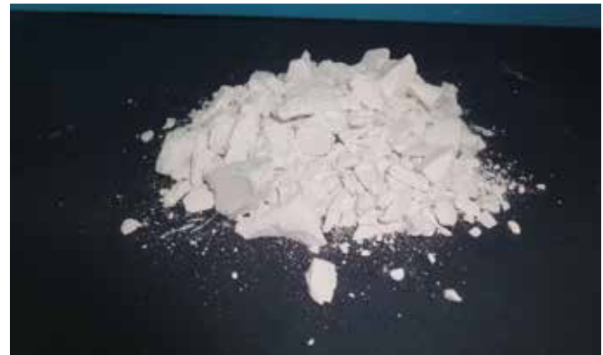
Bahan prabakar selepas proses pencampuran dan pengisaran basah Prefired material after mixing and wet grinding process
