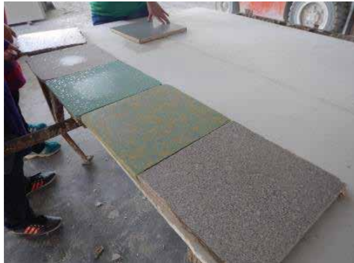
Marmar sintetik yang dihasilkan di industri Synthetic marble produced in industry
