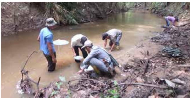
Persampelan kelodak dan konsentrat bagi kajian sumber pemineralan emas di Sg. Jenalik, Lanchang, Pahang Sampling of silt and concentrates for gold mineralization resource study at Sg. Jenalik, Lanchang, Pahang
