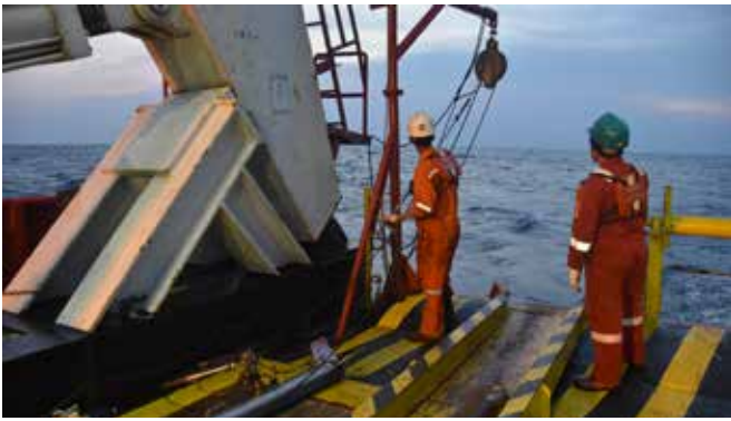
Sonar imbasan sisi dan boomer sedang diturunkan bagi melaksanakan survei geofizik Projek Kajian Sumber Pasir Laut Negara Fasa 3 – Lepas Pantai Pahang dan Johor Timur Deploying of side scan sonar and boomer for geophysical survey of National Offshore Sand Resource Study Phase 3 – Offshore Pahang and East Johore
