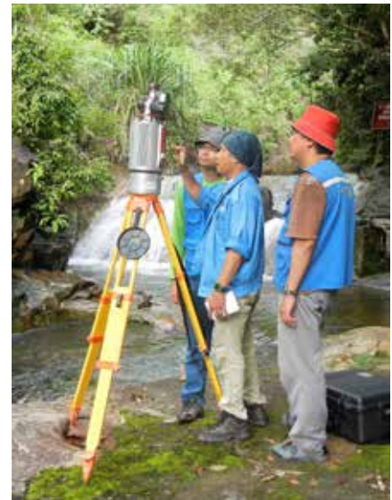
Pengukuran lokasi menggunakan real time kinematic GNSS di Gurun, Kedah Real time kinematic GNSS positioning measurement at Gurun, Kedah
