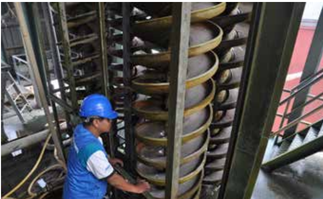
Pengeluaran mineral silika menggunakan kaedah “spiral” di Sungai Bakong, Marudi Sarawak Production of silica mineral by the spiral method at Sungai Bakong, Marudi Sarawak
