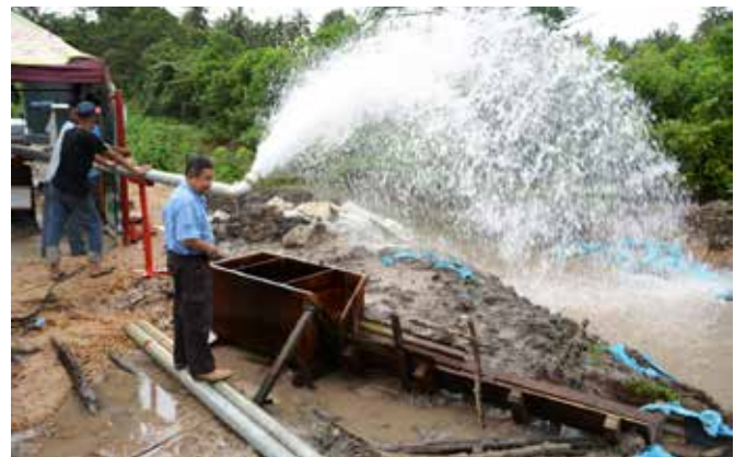
Ujian pengempaman di Sri Gondang, Bachok Kelantan Pumping tests at Sri Gondang, Bachok Kelantan
