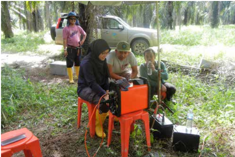
Survei keberintangan 2-D di kawasan Tasik Chini 2-D resistivity survey at Tasik Chini Area
