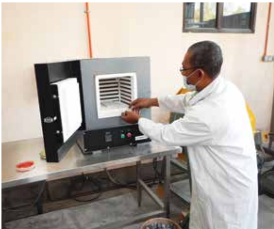
Proses pensinteran (700 - 800°C) Sintering process (700 - 800°C)
