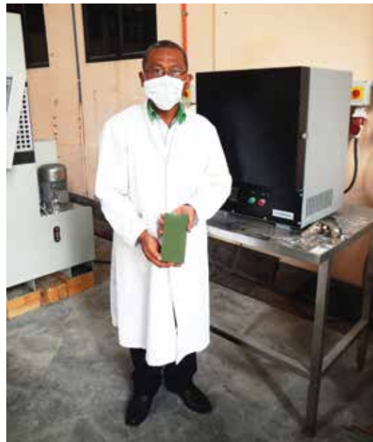
Sampel jubin kaca selepas proses pensinteran Glass tile samples after sintering
