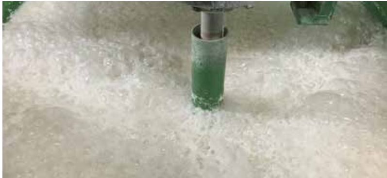
Penyediaan buburan pulpa berpengisi PCC Preparation of pulp slurry impregnated with PCC
