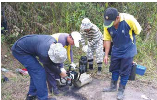
Pengerudian batu arang di Melikin, Serian, Sarawak Hand-drilling coal seam at Melikin, Serian, Sarawak
