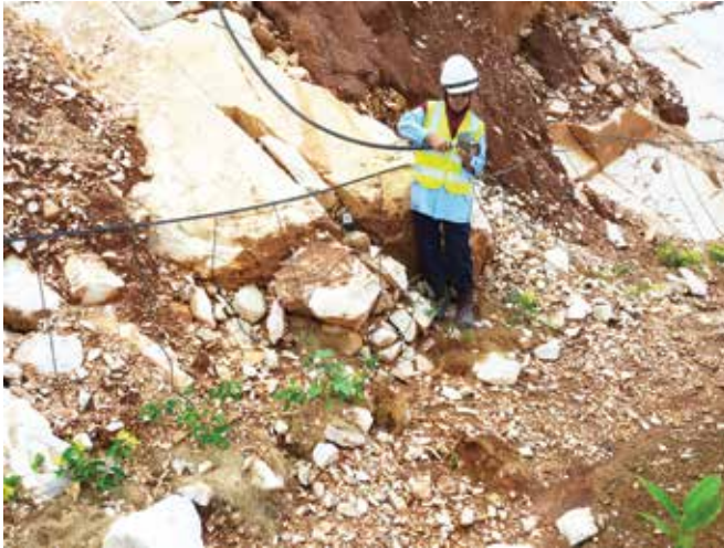
Aplikasi kaedah pengairan secara automatik di Kuari Imerys, Ipoh The application of automatic irrigation methods at Quarry Imerys, Ipoh
