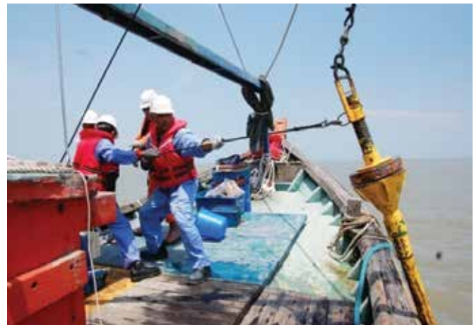
Persampelan teras dilaksanakan bagi Kajian Tumbesaran dan Kematian Kerang di Tapak Ternakan Kerang di Selangor Core sampling executed during The Study of Cockle Growth and Death at Cockle Farm offshore Selangor
