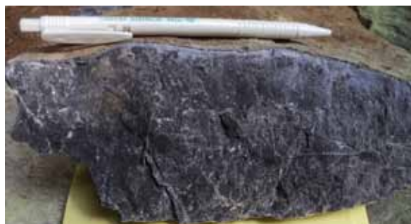
Batu kapur Formasi Setul berwarna kelabu gelap, bertekstur halus dan mengandungi mikro-teleraung kalsit serta tekstur stilolit dari kawasan Wang Kelian, Perlis. Grey colour and fine-grained limestone of Setul Formation with stylolitic texture and calcite veinlets from Wang Kelian area, Perlis.
