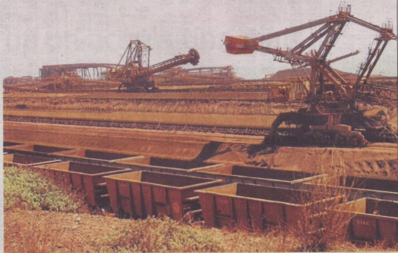
Market demand: Stackers and reclaimers moving iron ore to rail cars at Rio Tinto's Port Dampier operations in Western Australia's Pilbara region. The global market is in a state of flux, with lower-grade ore increasingly shunned in favour of better-quality material. — AFP
